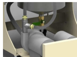
Slurry Pump and Polyurethane Joint
