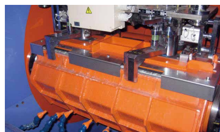
蓋の開閉機構 / Structure of Opening and Closing of Barrel Lid
