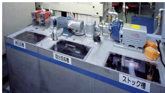
Polymer coagulating tank and coagulating sedimentation tank are not required, which are required by conventional coagulating sedimentation equipment.
