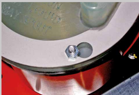
ダルマ孔 / key - hole - shaped holes
